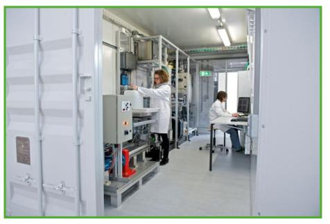
Figure 3: Mobile KONTI-C pilot plant for on-site gasification/methanation of wet biomass. The KONTI-C pilot plant will be part of the Energy System Integration platform at PSI.
