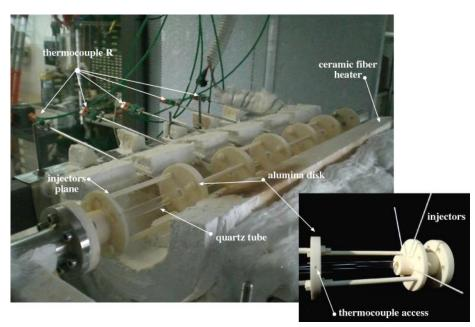
*Figure 2: MILD combustion: tubular reactor and mixing section, Istituto Ricerche sulla Combustione - CNR.*
