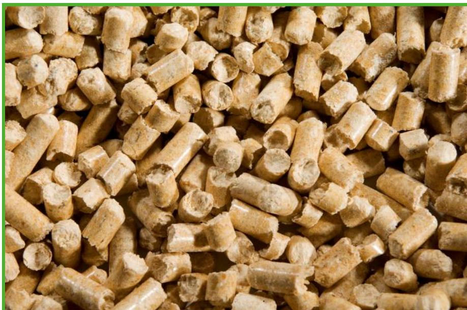
*Figure 1: A1-class wood pellets according to EN ISO 17225-2 standard.*
