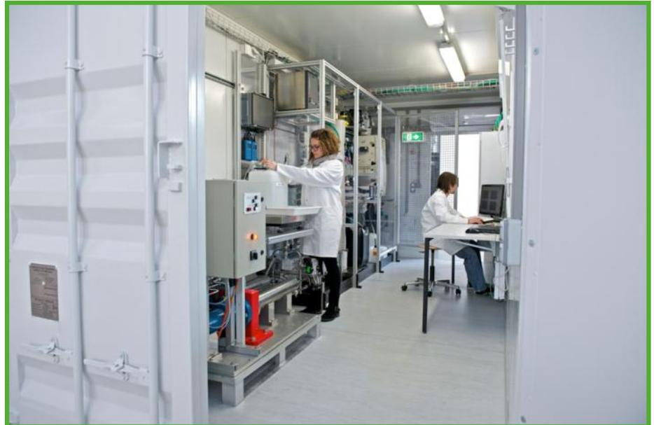
*Figure 3: Mobile KONTI-C pilot plant for on-site gasification/methanation of wet biomass. The KONTI-C pilot plant will be part of the Energy System Integration platform at PSI.*
