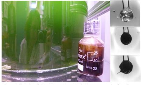
Figure 1: Left - Pyrolysis oil from algae, CIRSA Ravenna – University of Bologna; Right - Combustion phases of the algae pyrolysis oil, Istituto Motori - CNR.
