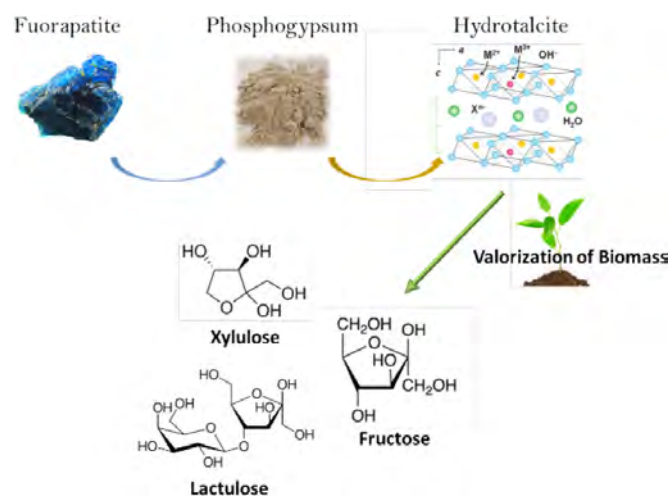
Figure 1: Schematic representation of PG-derived hydrotalcite-type catalysts for the valorization of biomass derivatives (i.e. sugars isomerization)
