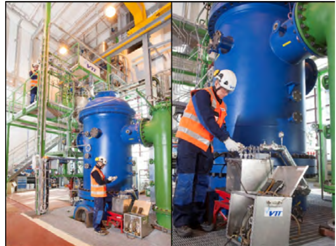
Figure 2: VTT's one-megawatt pressurized fixed-bed gasification pilot plant (SXB-Pilot) in Finland (VTT)
