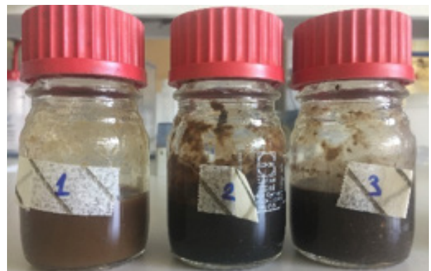
Figure 1: On the left, dehydrated sewage sludge. On the right, sewage sludge hydrolysate
