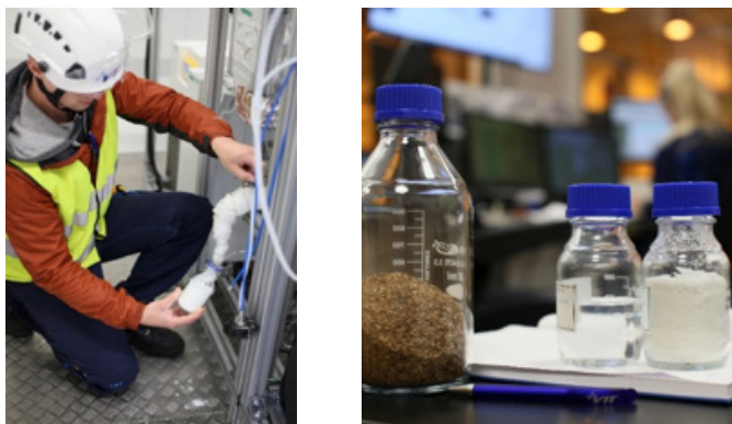
Figure 1: Collecting FT-wax from the synthesis unit Mobsu - on the right: crushed bark (woody raw material for gasification), FT liquid product and FT wax
