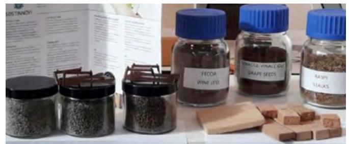
Polypropylene and clay bricks samples produced with waste material from the wine production chain
