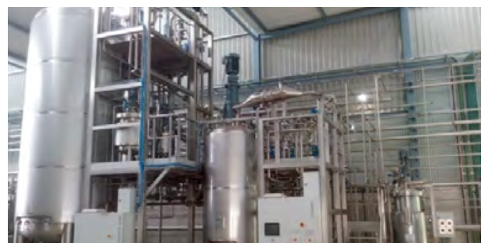
Fermentation train of the Mid-stream unit: 300 l, 3,000 l and 20,000
