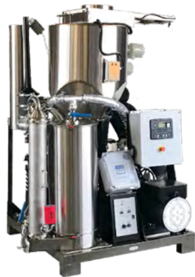
Small Scale PP20 APL Gasifier
