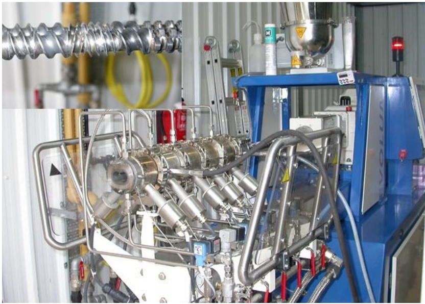
Figure 1. Twin-screw extrusion equipment at CIEMAT facilities and detail of screw configuration inside the barrels.
