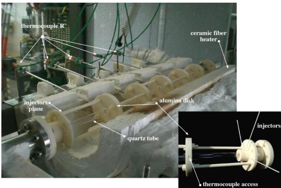
Figure 2: MILD combustion: tubular reactor and mixing section, Istituto Ricerche sulla Combustione - CNR.
