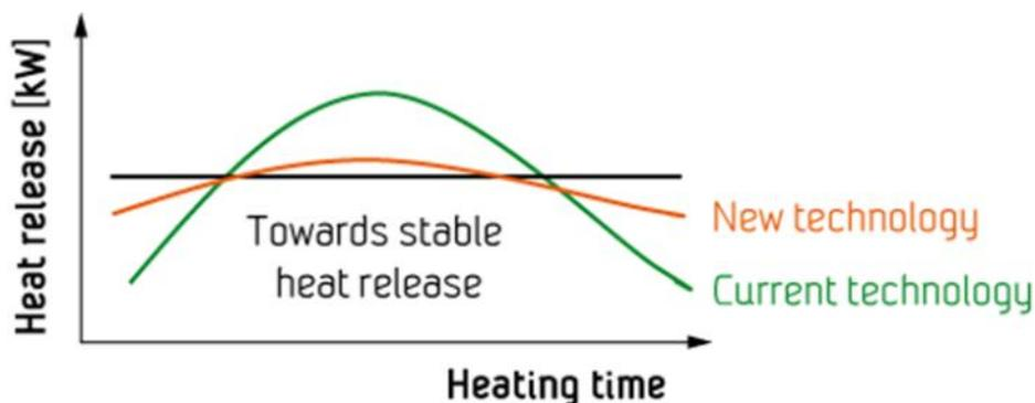
**Figure 1: SINTEF StableWood project.** This diagram illustrates the lower heat release peak and more stable heat release most adapted to the well-insulated residential buildings of tomorrow.
