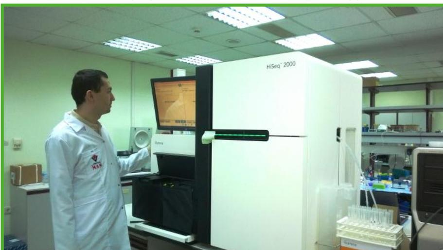
Figure 3: Illumina HiSeq2000 sequencing platform at TÜBİTAK Marmara Research Centre (MRC) Genetic Engineering and Biotechnology Institute.
