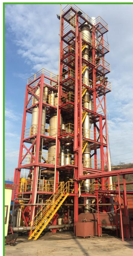
**Figure 1: Chinese 10000 t/y CFB fast pyrolysis demonstration plant in Shanxi.**
